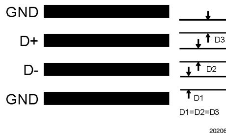
FIGURE 9. Ideal Diode Trace Layout
